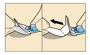
**7a.** Remove adhesive pad liner. Hold the sensor in place and gently remove the adhesive liner from under the adhesive pad. Do not remove the liner on the rectangular adhesive tab yet.
