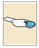
**8a. Untuck** adhesive tab. Untuck the adhesive tab from under the sensor connector.
